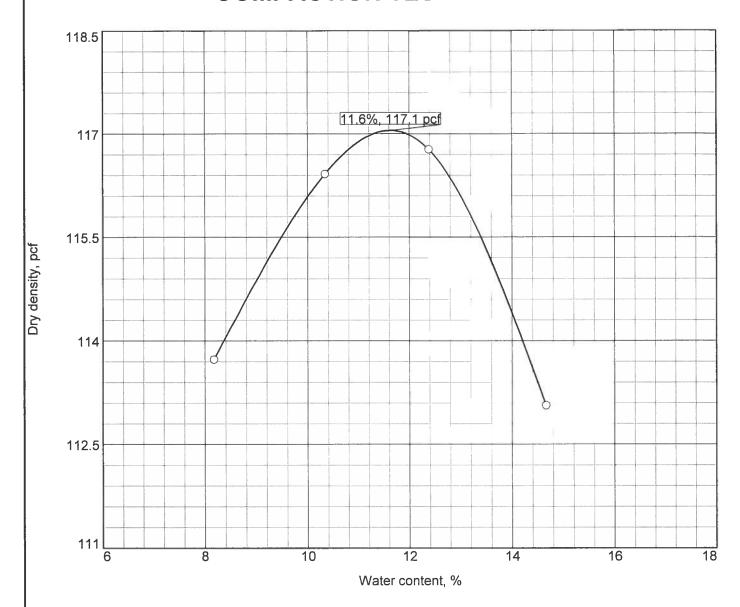
Test specification: ASTM D 1557-02 Method A Modified
