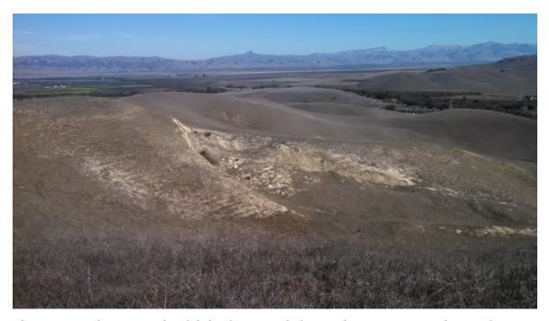
Photo 4 – Moderate size landslide along south facing slope. View is to the northeast. Note how slide extends below surficial soils.
