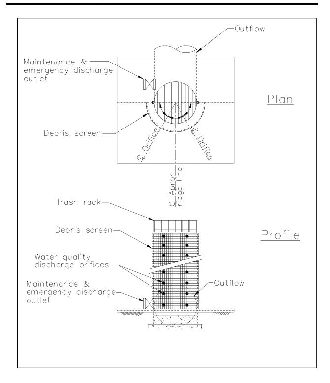
FIGURE 2: MULTIPLE ORIFICE OUTLET RISER
