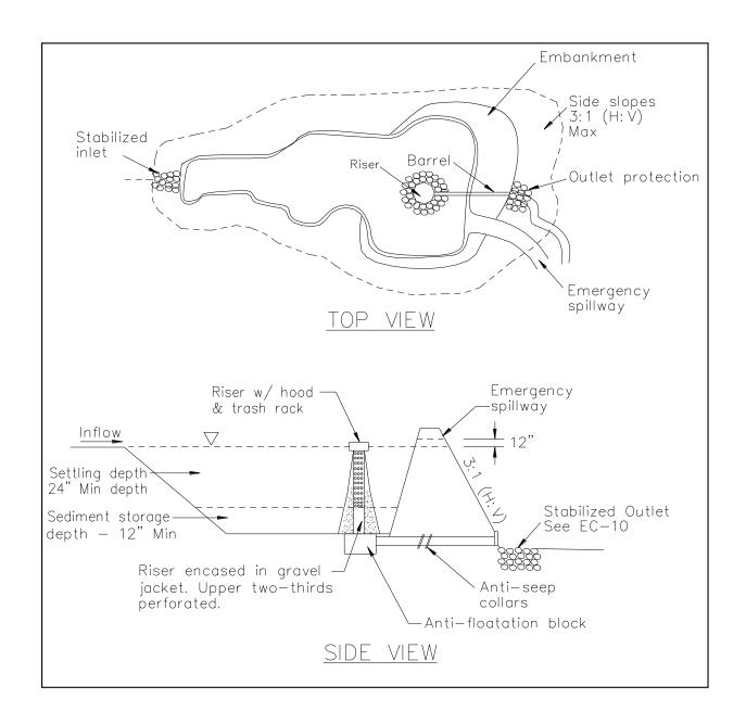
FIGURE 1: TYPICAL TEMPORARY SEDIMENT BASIN
