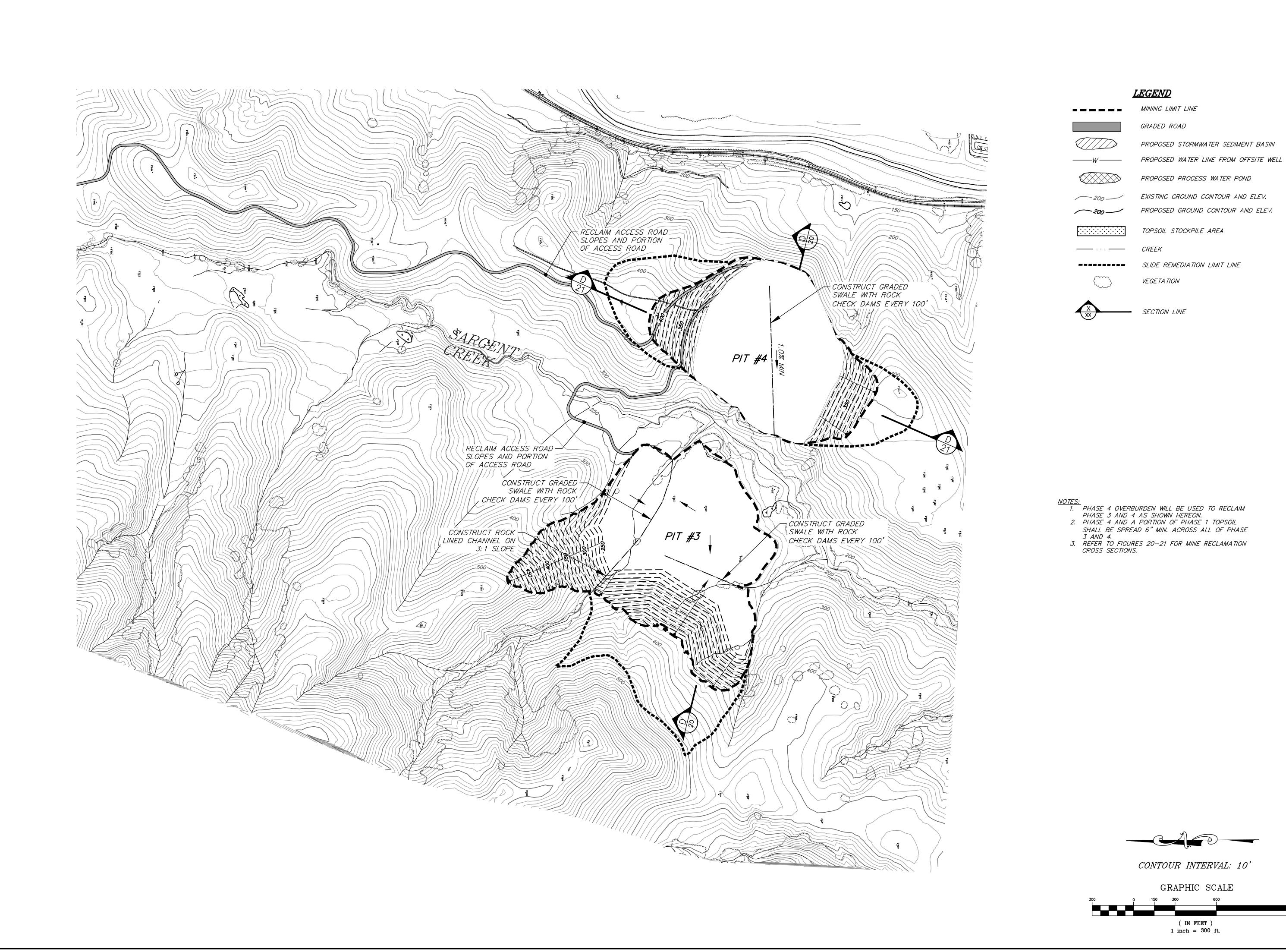
PROPOSED STORMWATER SEDIMENT BASIN
