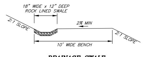
DRAINAGE SWALE *NO SCALE*
