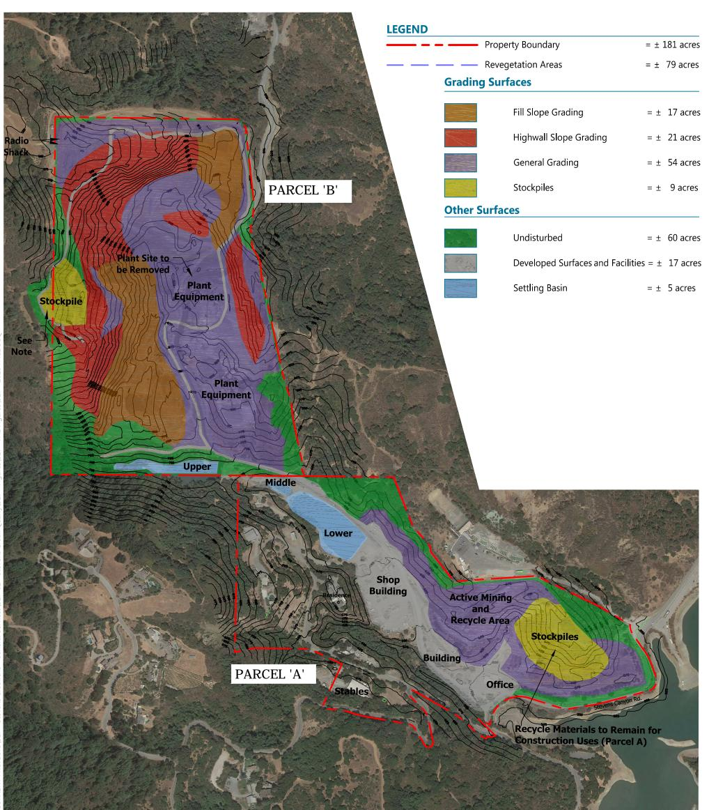
TOPOGRAPHY SOURCE: Aero-Geodetic Corporation (2006-10-26) CONTOUR INTERVAL: 25'-0" AERIAL IMAGE SOURCE: Google Earth Pro (2018-08-09) NOTE: Western offsite encroachment received prior consent and is addressed in prior
