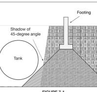
FIGURE 7-1 7.2.4.1. Ensure that downward forces from loads carried by the foundations and supports of nearby structures (constructed before or after tank installation) are not transmitted to the tanks.
