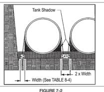
7.5.2. SPACING IN STABLE IN SITU (NATIVE) SOIL CONDITIONS 7.5.2.1. The minimum spacing between the sidewall or endcap of the tank and the side of the excavation must be 18 inches. See FIGURE 7-3.
