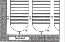
FIGURE 7-3 7.5.2.2. If two or more tanks are installed in the same hole, allow for at least 18 inches between the tanks. See FIGURE 7-3. 7.5.2.3. If two or more tanks are installed in the same hole and equal to or greater than two times the width of the deadman or deadmen required between the tanks. See FIGURE 7-2 and
