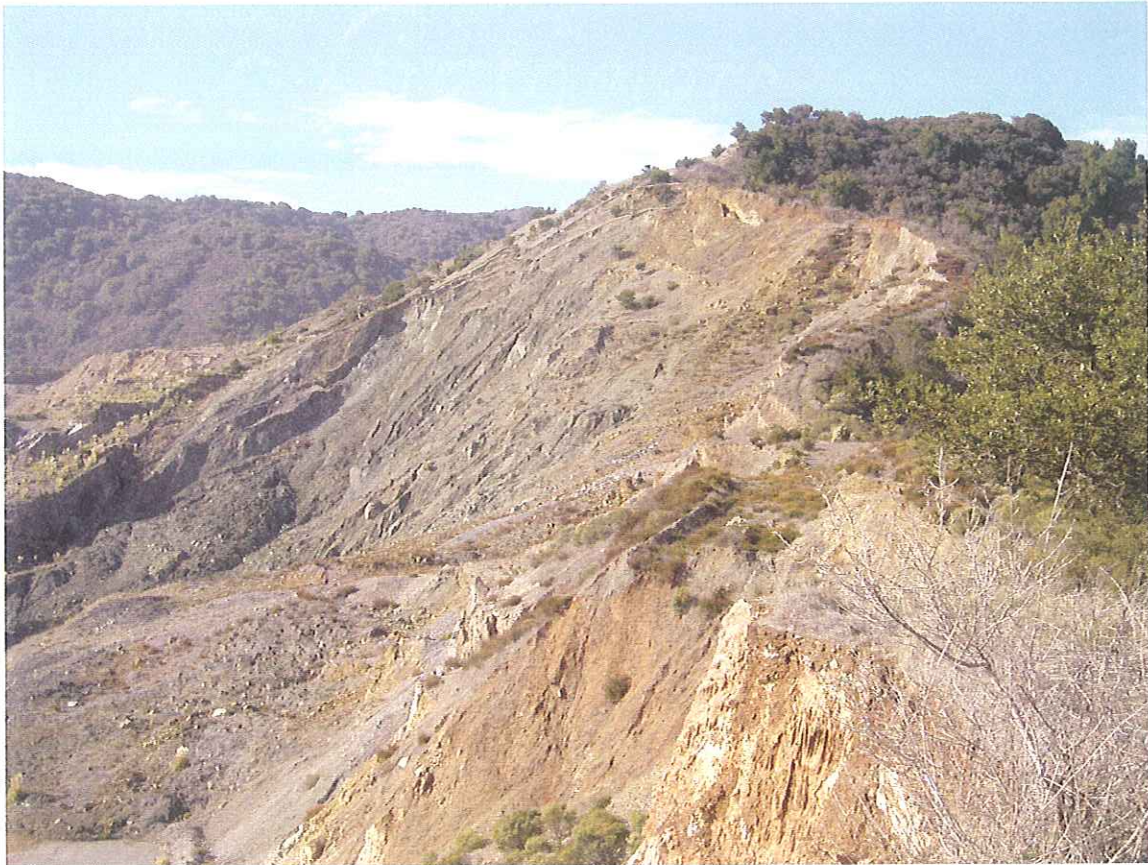
Photo 2. The Main Landslide showing well-defined scarps above the "headscarp" area, indicating ongoing deep-seated failure of the upper portion of the landslide.
