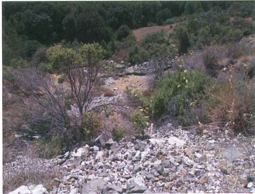
Photo 9: Looking downslope from rockied outfall shown in Photo 8 at silt fencing and area where soil mixed with talus was observed in 2012, 2013 and 2014 that may be the result of past slide; silt fence shows no visible significant displacement. Dated September 3, 2015.
