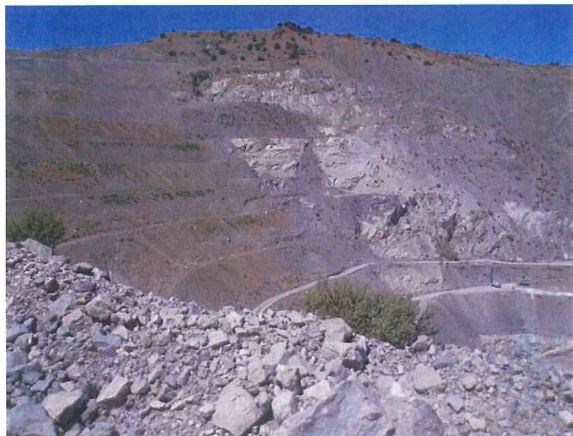
Photo 2: North Quarry western highwall with backfill. Dated September 3, 2015.
