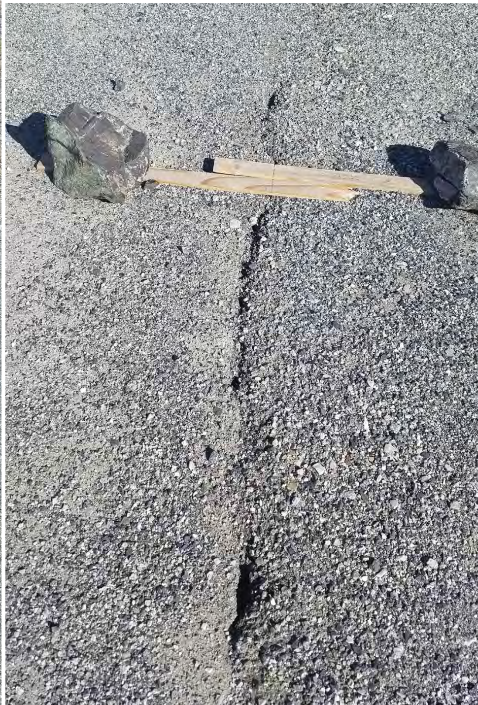
Photos #30A, B and C – Recently formed ground cracks near eastern portion of Yeager Yard slide. (Monitoring sticks placed by Operator.)
