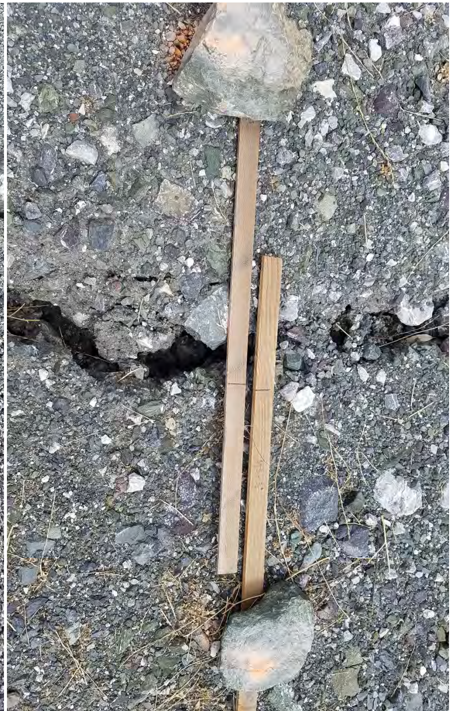
Photos #30A, B and C – Recently formed ground cracks near eastern portion of Yeager Yard slide. (Monitoring sticks placed by Operator.)
