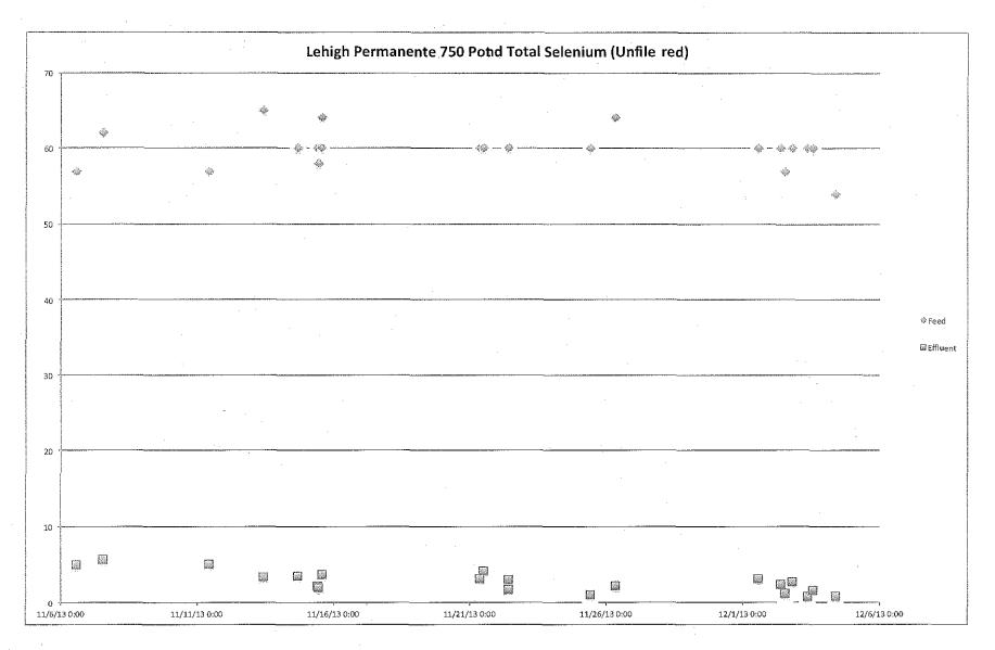
Note: Feed water concentrations were artificially elevated due to low selenium in quarry well water.
