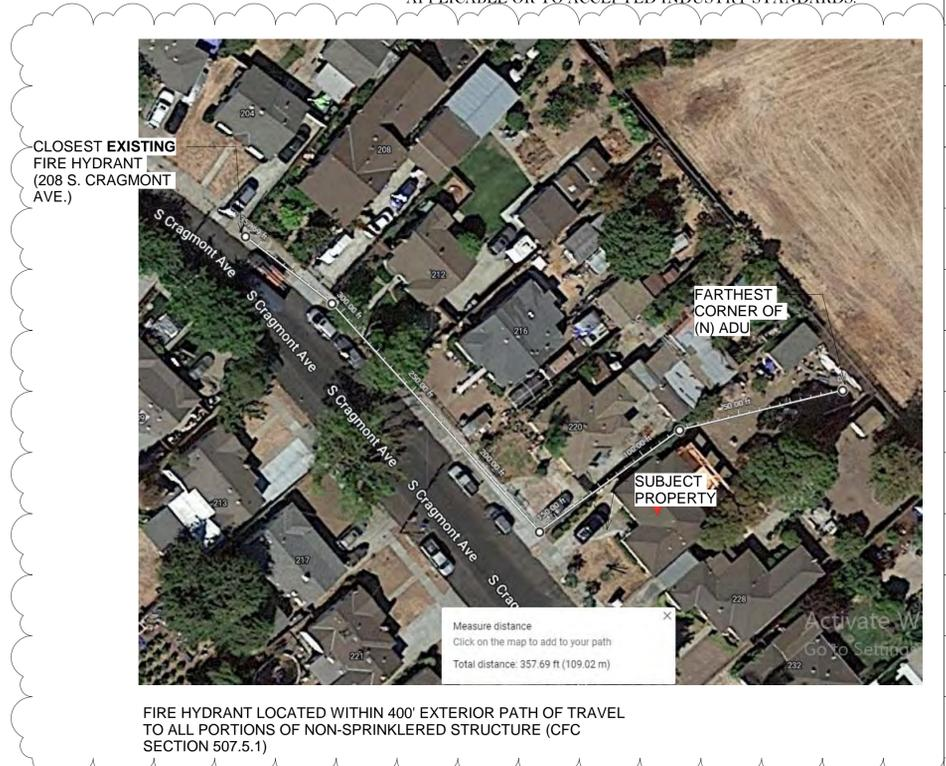
FIRE HYDRANT LOCATED WITHIN 400' EXTERIOR PATH OF TRAVEL TO ALL PORTIONS OF NON-SPRINKLERED STRUCTURE (CFC SECTION 507.5.1)
