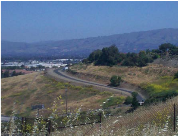
PHOTOS 3, 4: Design access roads and driveways to follow natural grade, contour and topography.
