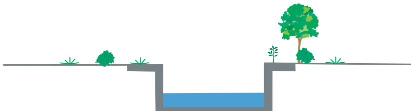
D. Concrete lined channel
