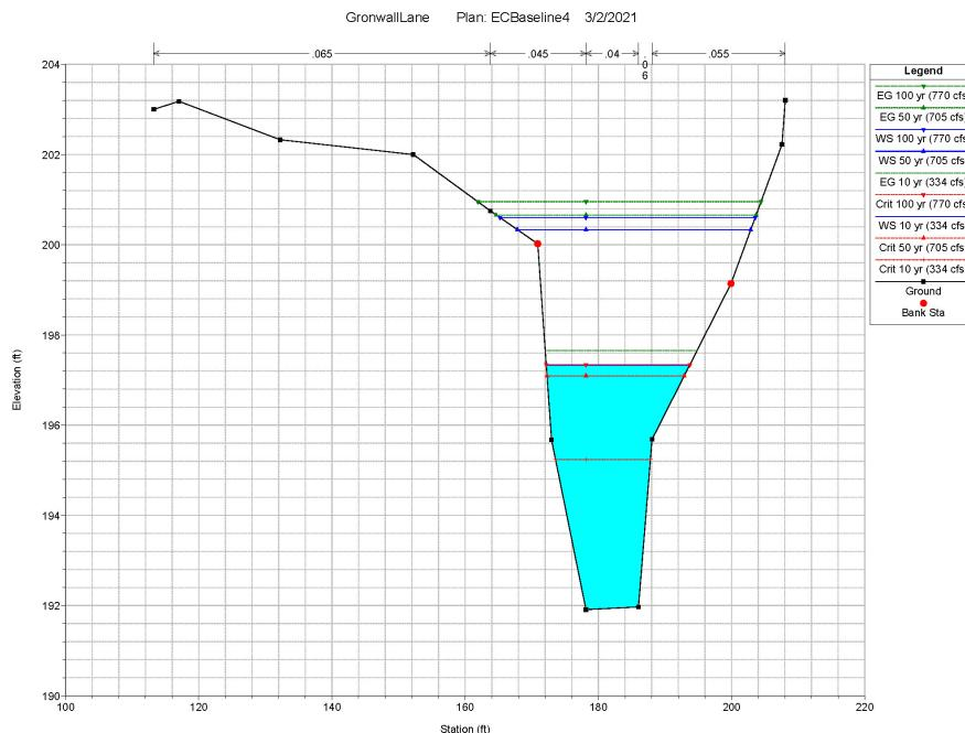
As denoted by gray fill in Table 3, existing conditions roughness values assigned to the poorly vegetated and moderately vegetated bank surfaces within the 100-foot-long planting plan area were 0.045 in the upstream 65 feet and 0.055 in the downstream 35 feet, according to field inspection. Figure 1 shows the existing conditions model cross-section at STA 13+90.
