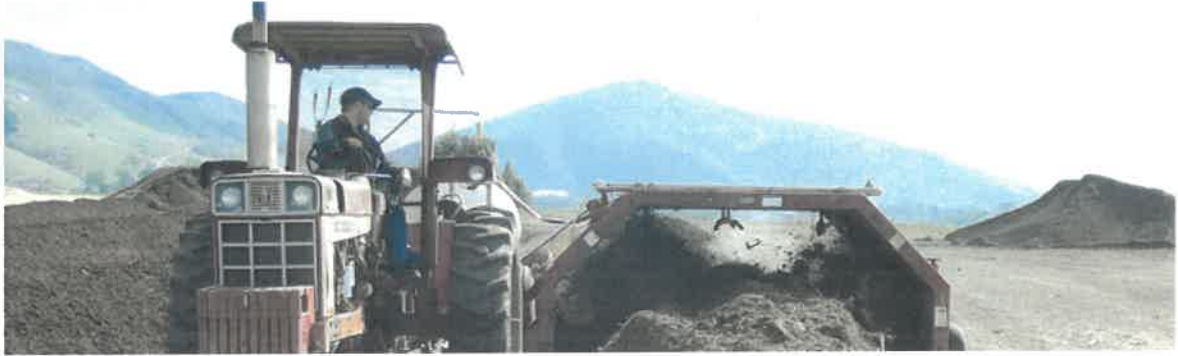
Figure 7: Windrow turner at Cal Poly compost facility
