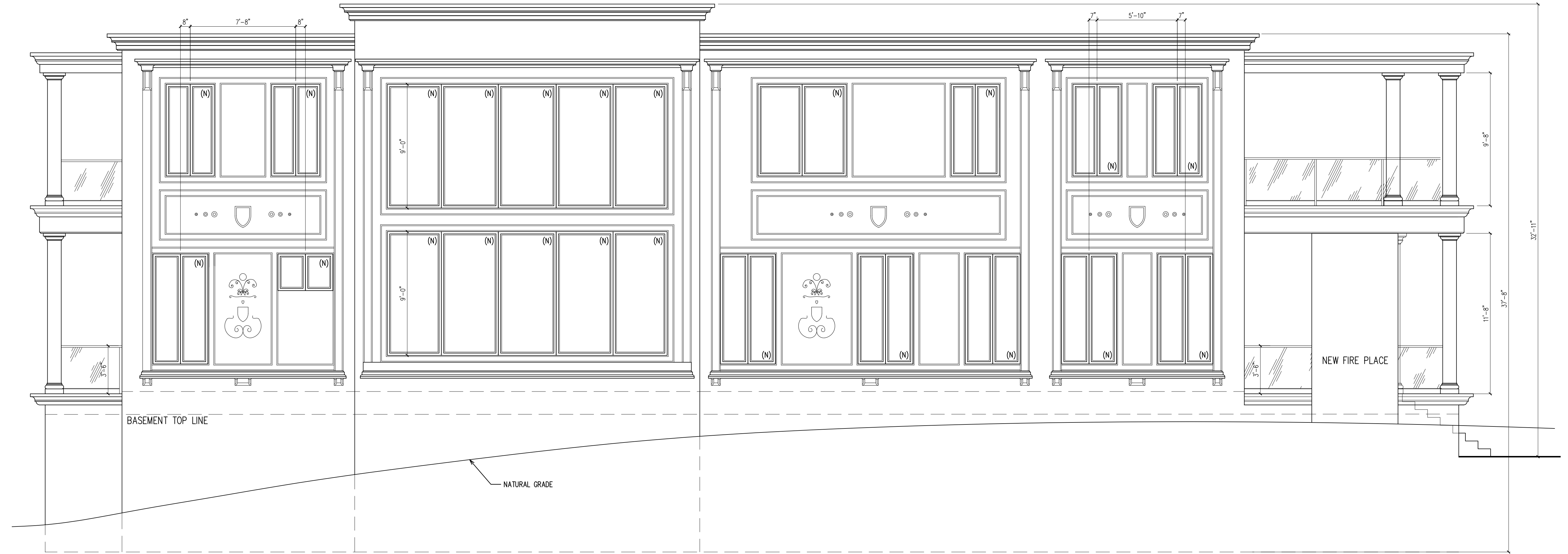
② PROPOSED BACK ELEVATION 1/4" = 1'
