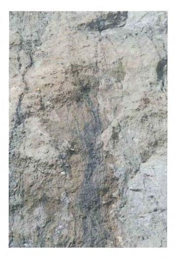
Photo 12: A close-up of the right seep shown in the previous photograph. Note the gray clay seam below the water entry point
