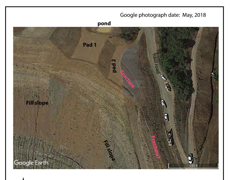
This is an enlargement of the photograph in figure 9. The fractures extend from the east side of Pad 1, across Pad 2 and curve south along the top of the east fill prism. The northern end of of the two fractures is easy to see, but their southern extent is unclear (hence the ?).
