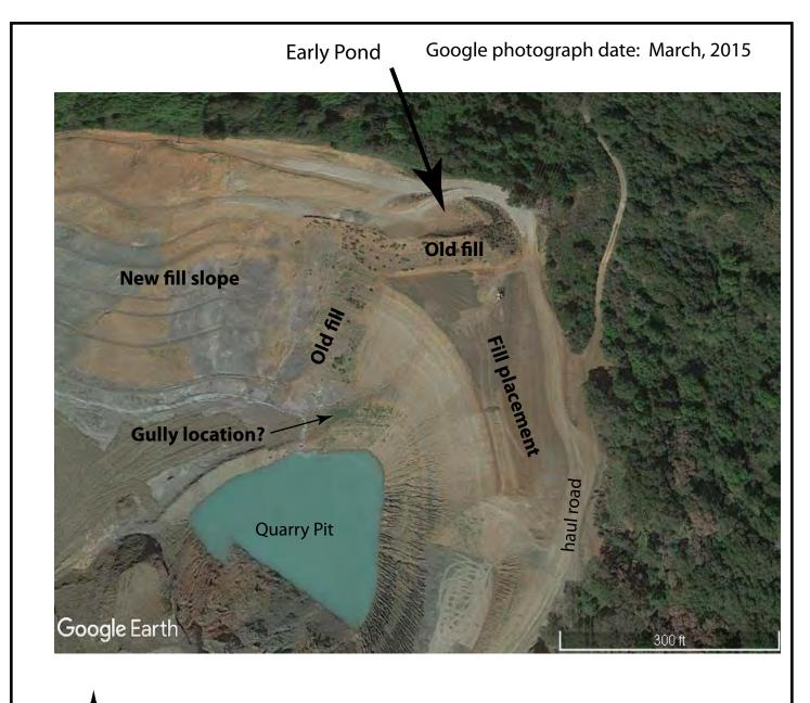
The fill prism on the east face has continued to grow. Only small areas of old fill in the NE corner remain exposed. The gully is completely covered. It appears that a pond or pad had been constructed at the top of the NE quarry corner.
