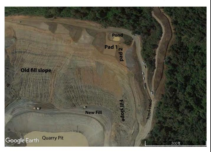
The quarry has deepened. Fractures have developed along the south edges of pads 1 and 2 (see next figures).
