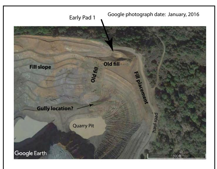
The eastern fill prism has grown higher. The face of the east fill prism is steep. A green area is visible at the toe of the slope where the east and north fills connect (the toe of the gully). The green area indicates that water is collecting in this area. The photo was taken in January and it is likely that surface water is concentrating in this area.
