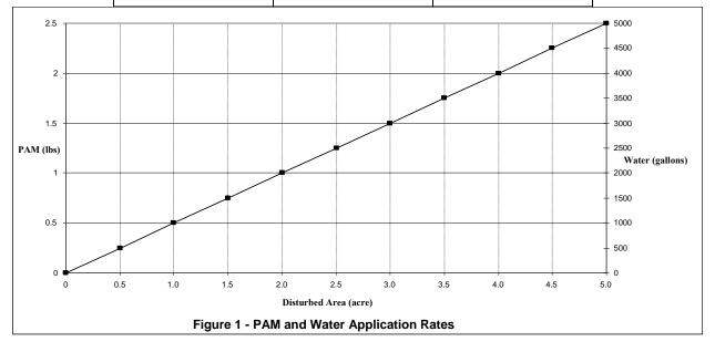
Pre-measure the area where PAM is to be applied and calculate the amount of product and water necessary to provide coverage at the specified application rate (1/2 pound PAM/1000 gallons/acre).
