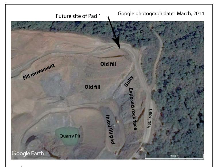
This photo shows the quarry soon after mining of the eastern face stopped (labeled - exposed rock). New fill is beginning to be placed along the base of the east face (initial fill pad). Note the gully that marks the junction between exposed rock and the old fill that had been placed on the north face. As fill was placed in this corner of the quarry, the gully formed a buried valley and a focus for groundwater.
