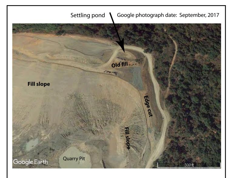
Fill continued to be placed on the north slope. Fill was removed from the base of the east slope (note the new quarry pit), and the top of the east face fill prism has narrowed slightly (see fill configuration on Figure 6.
