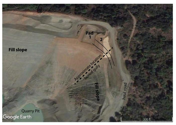
These are the physical relationships just prior to when the fractures formed (winter of 2017-18). The fractures occurred at the crest of the slope and define the zone of movement. The fill above the buried gully is at its the thickest when compared to either side (see Figure 2). This section of the face also has its steepest historical slope because fill was removed from the base of this slope (compare with Figure 6).
