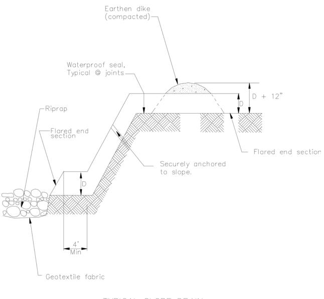
TYPICAL SLOPE DRAIN NOT TO SCALE
