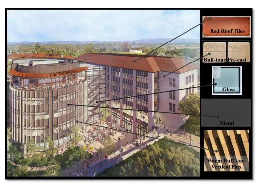
Figure 30 Bridge Building Elevations with Material Palette, Source: LMN Architects & UA/CPD
