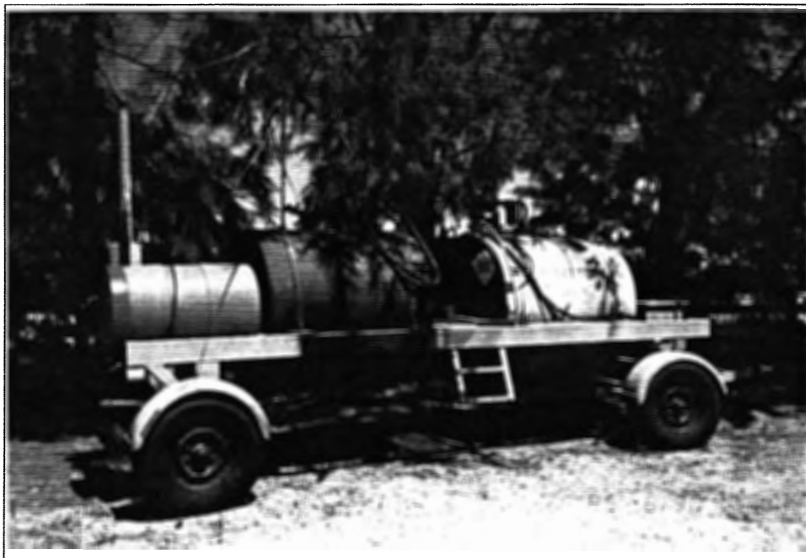
FIGURE 3B. VIEW OF TWO 500-GALLON PORTABLE ASTs, NEAR THE OLD MILK HOUSE, WHICH CONTAIN GASOLINE AND DIESEL.
