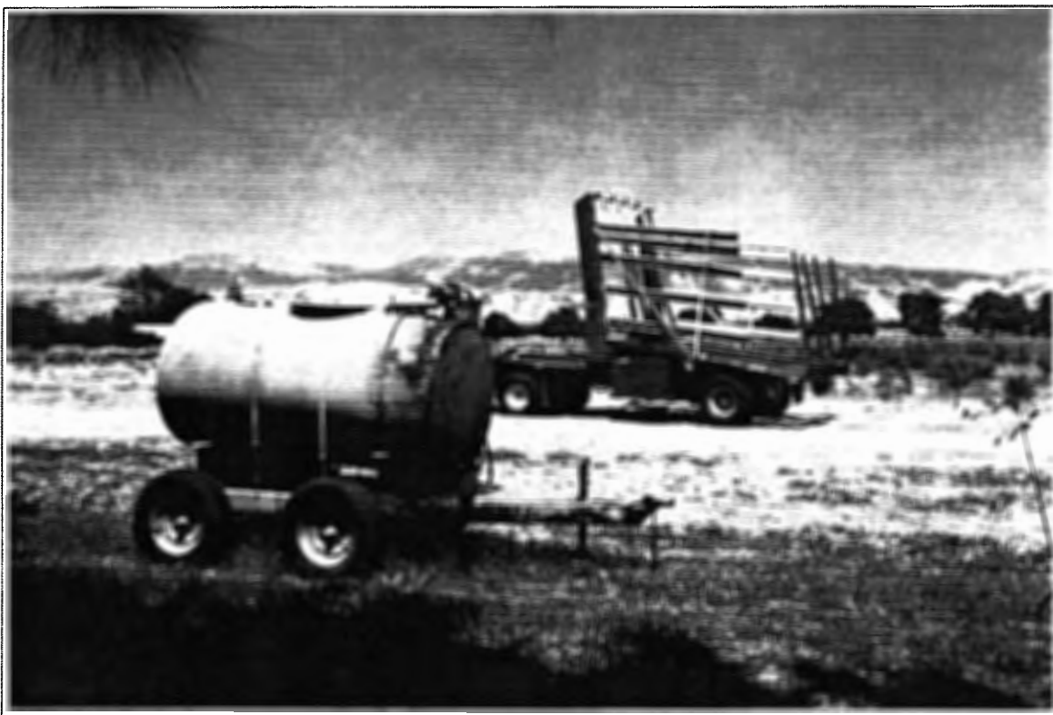
FIGURE 3A. VIEW OF ONE 500-GALLON PORTABLE AST IN THE HAY FIELD, WHICH CONTAINS GASOLINE.
