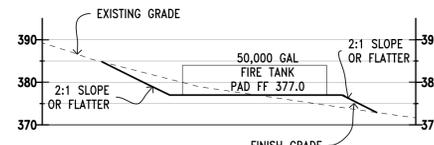
WATER TANK CROSS SECTION P-P
