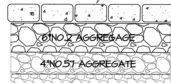
TYPICAL DETAIL PERVIOUS PAVERS PRIVATE DRIVEWAY NO SCALE
