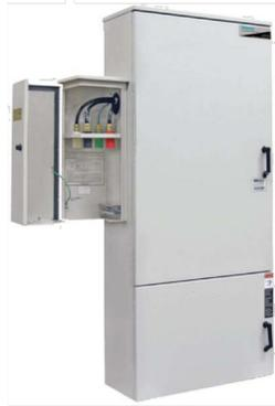
The AA-CL-T-3S Series also features a Square D load center; Strikesorb® surge suppression; a utility voltage sensing relay; a Cam-Lok style engine generator connector panel, mounted on the left or right; and a ground fault circuit interrupter (GFCI) circuit breaker wired to a duplex outlet in the Telco chamber.
