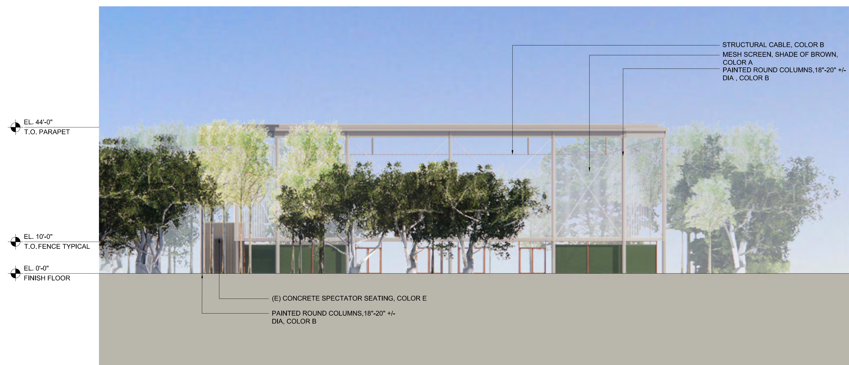
1 EAST ELEVATION (VIEW FROM KNIGHT MANAGEMENT CENTER) 1/16"=1'-0"
