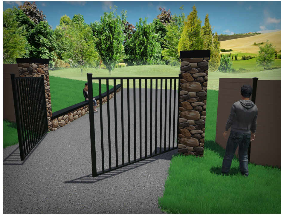
24 in. Square x 6'-8" tall, Steel, Masonry, Block, & Concrete, Columns. (see cross-section below)
