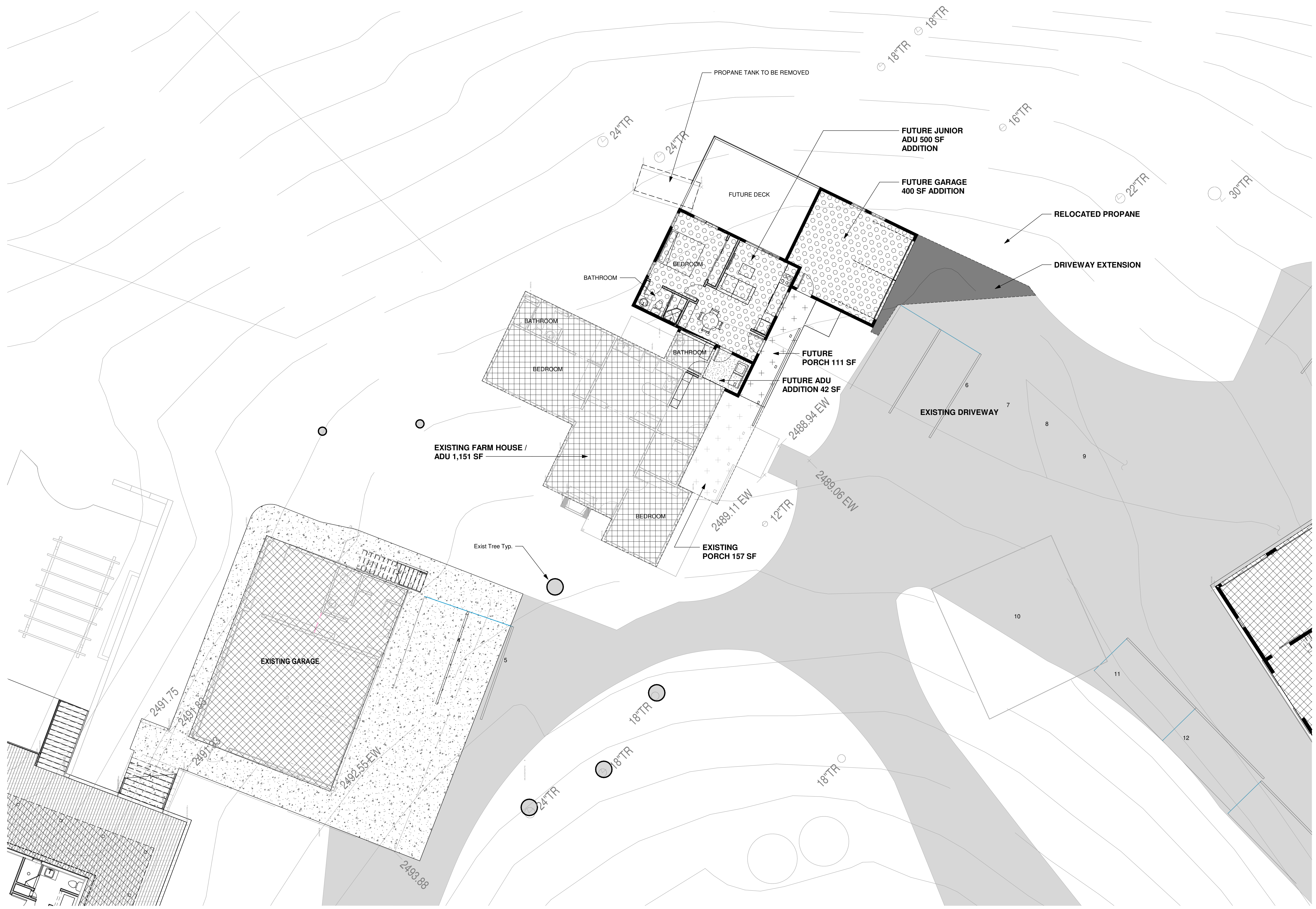
1 ENLARGED SITE PLAN FARM HOUSE (ADU) ADDITION OF JUNIOR ADU 1/8" = 1'-0"
