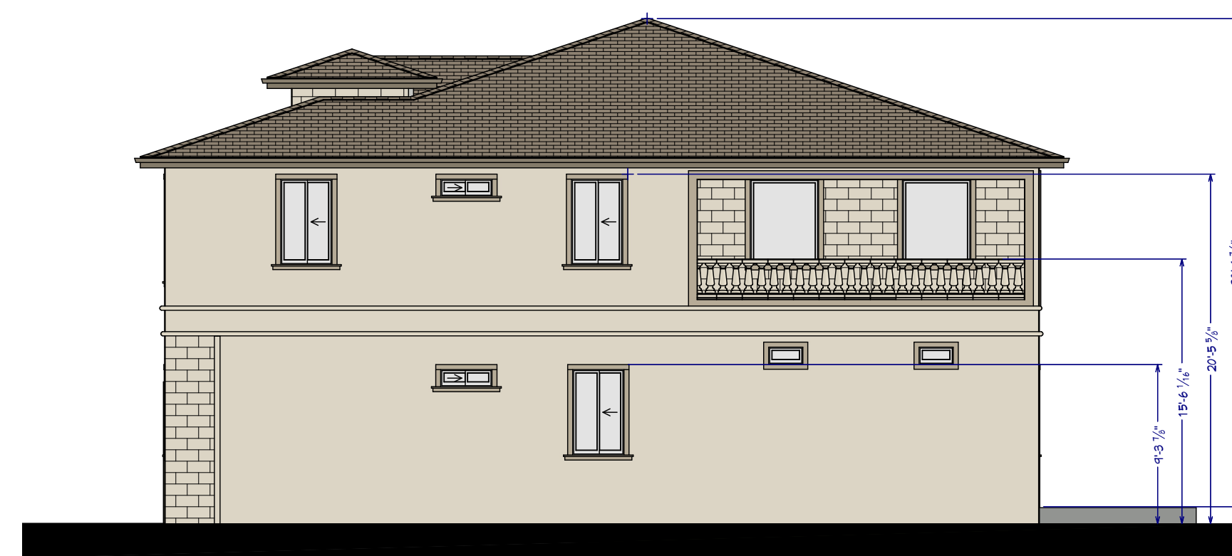
E4 EXTERIOR ELEVATION RIGHT 1/8 IN = 1 FT
