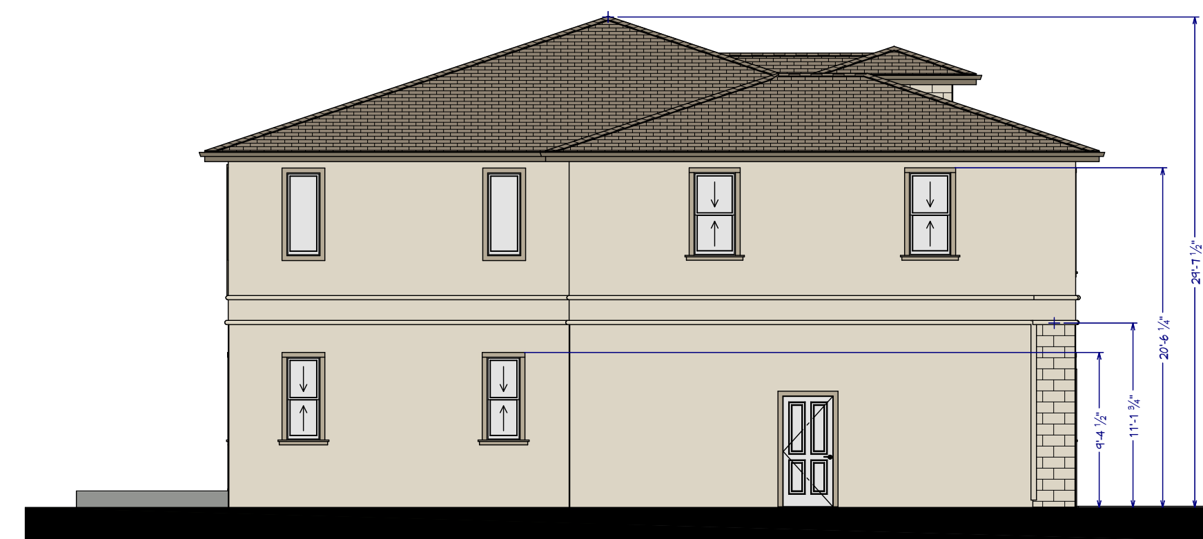
E2 EXTERIOR ELEVATION LEFT 1/8 IN = 1 FT
