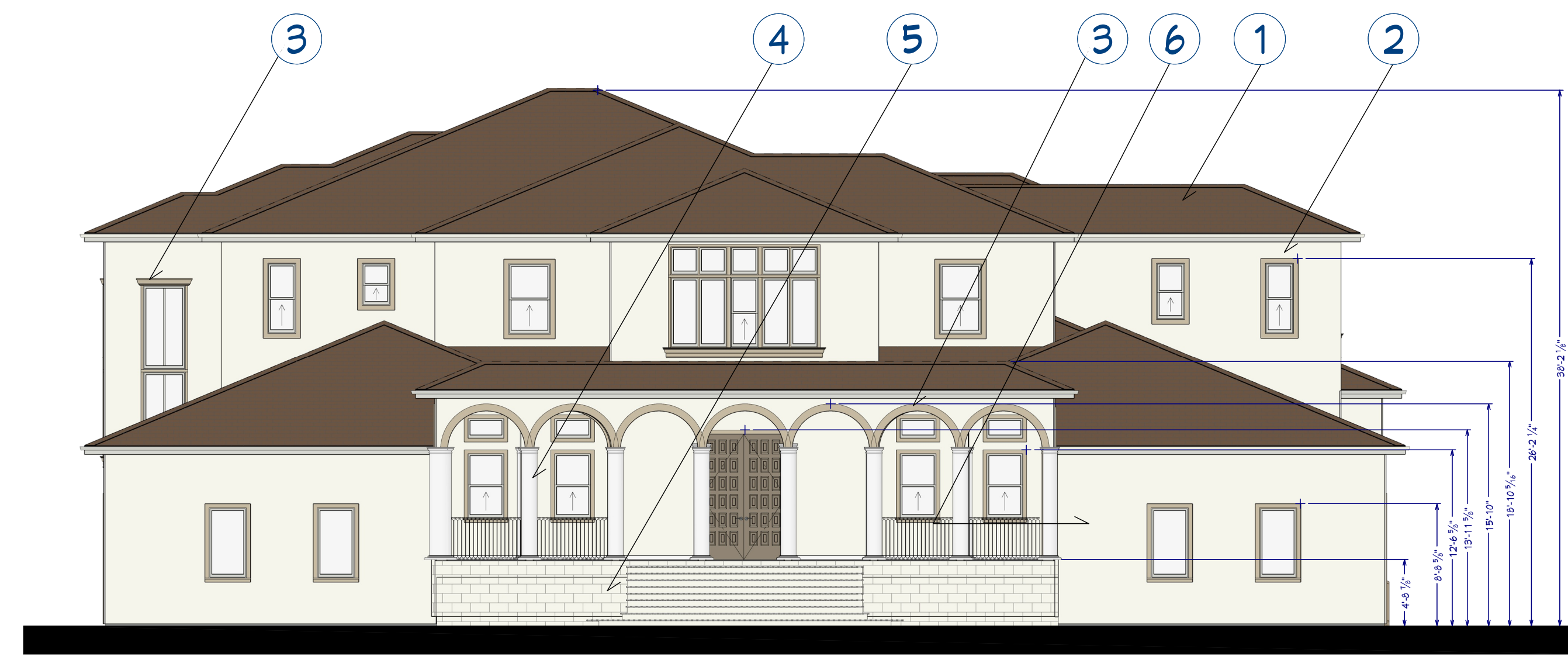
E4 EXTERIOR ELEVATION FRONT 1/8 IN = 1 FT
