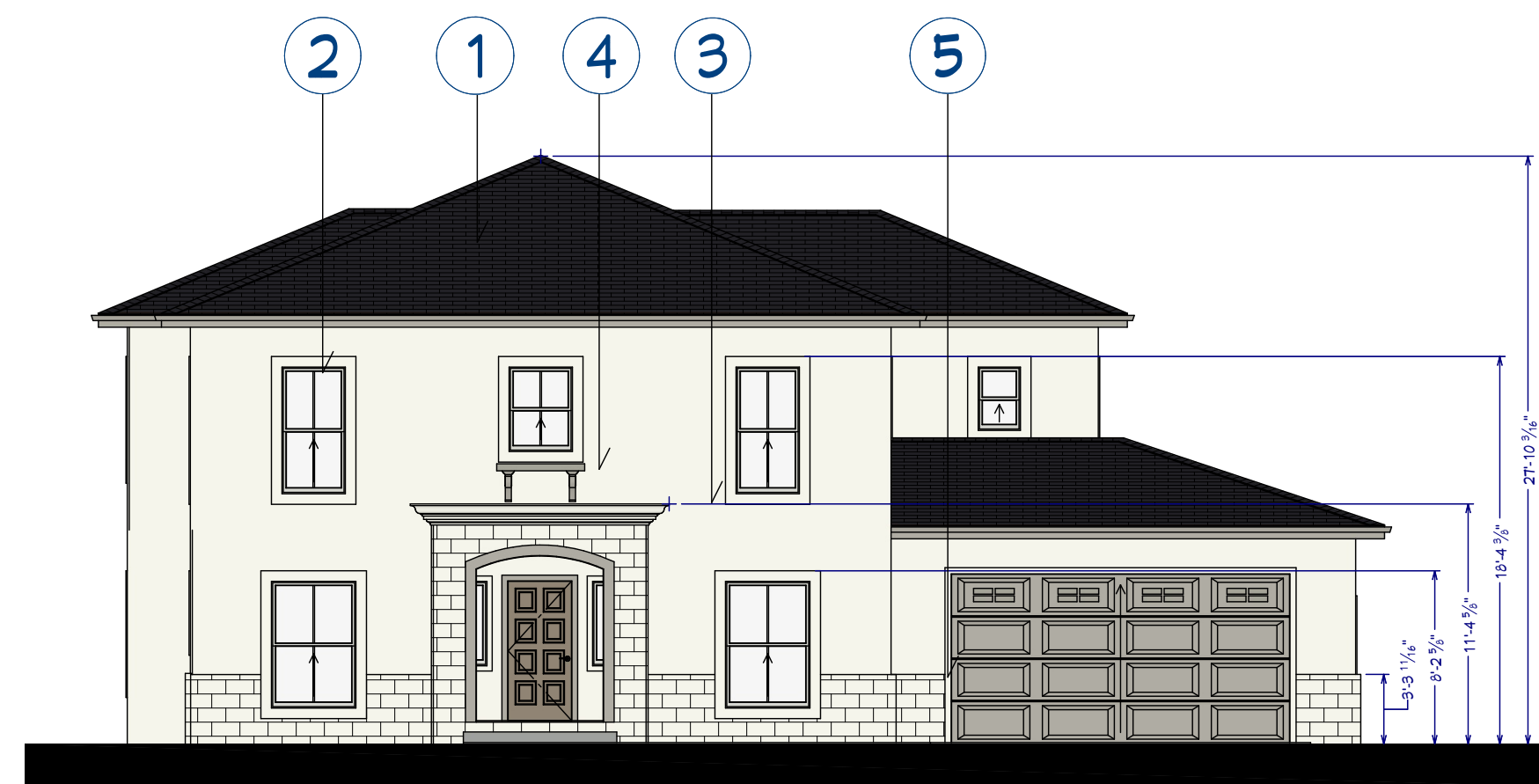
E1 EXTERIOR ELEVATION FRONT 1/8 IN = 1 FT
