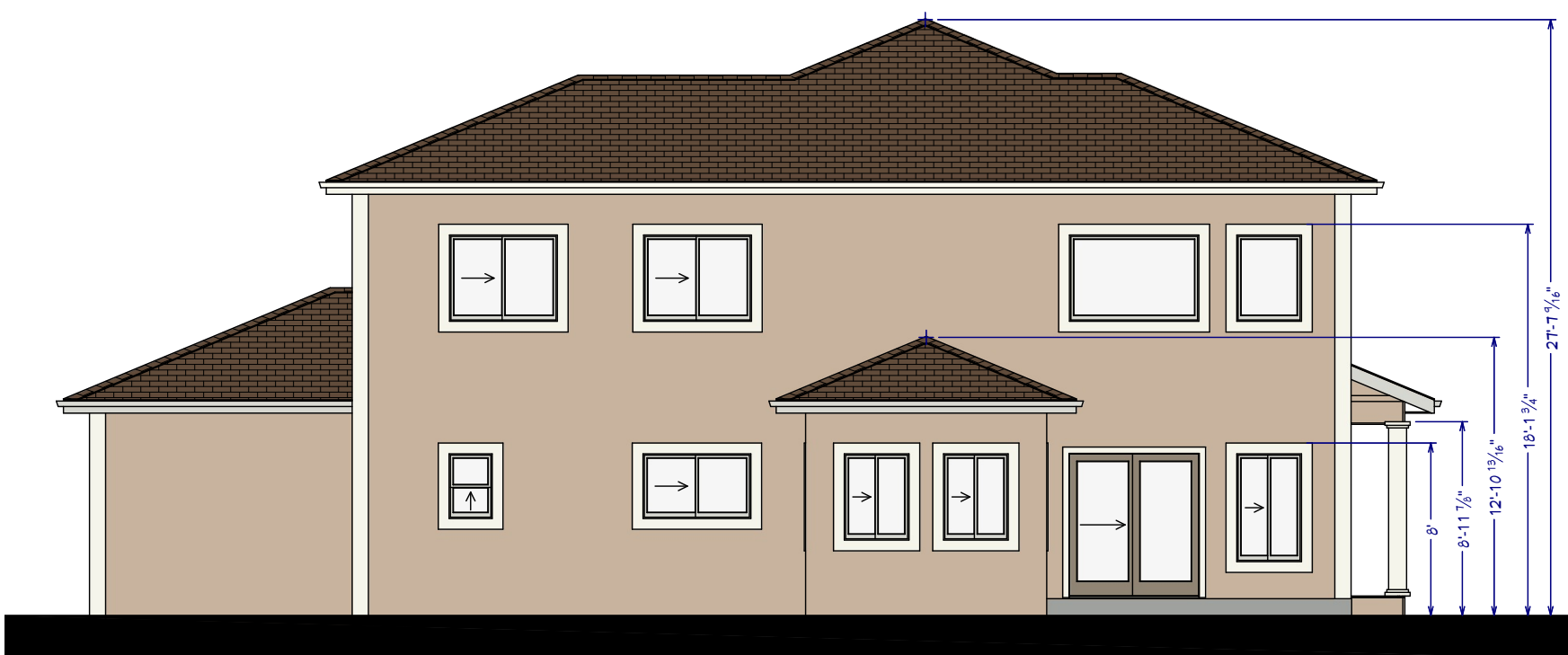
E3 EXTERIOR ELEVATION BACK 1/8 IN = 1 FT
