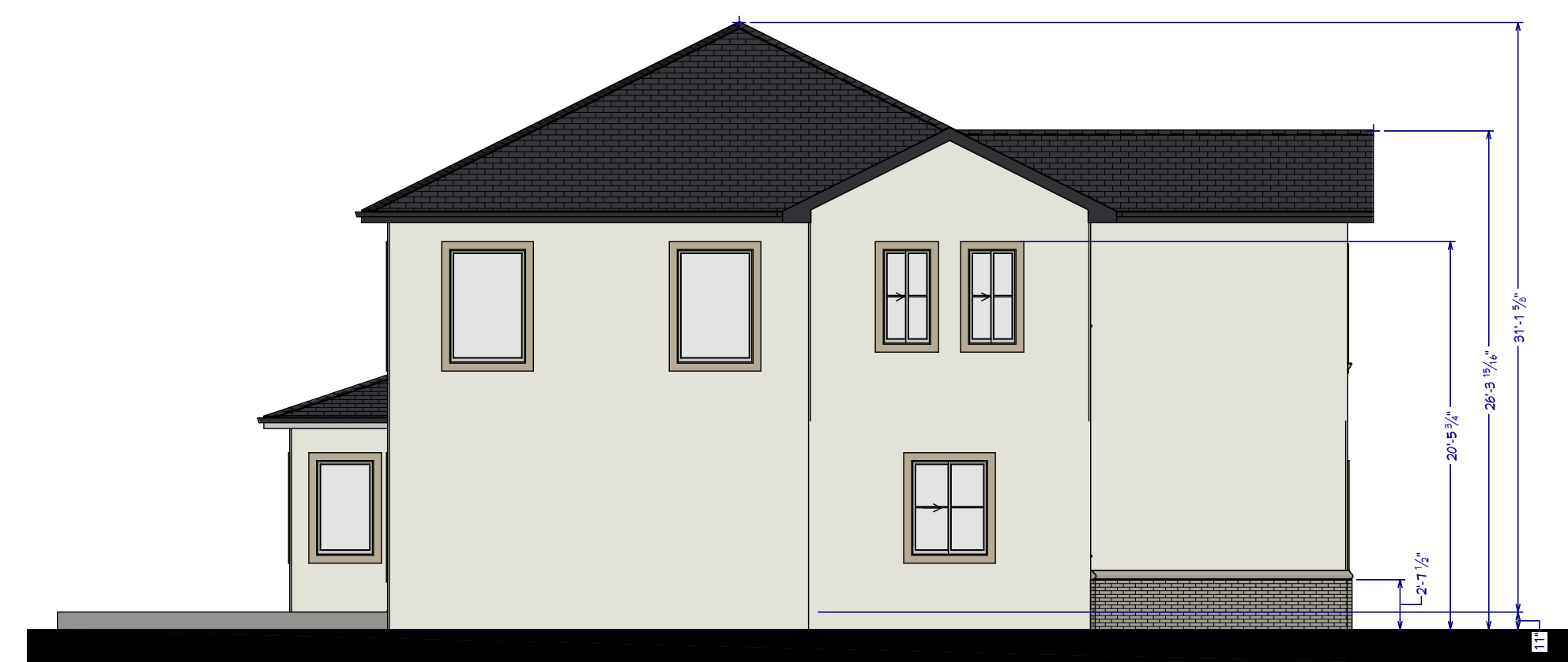
E2 EXTERIOR ELEVATION LEFT 1/8 IN = 1 FT
