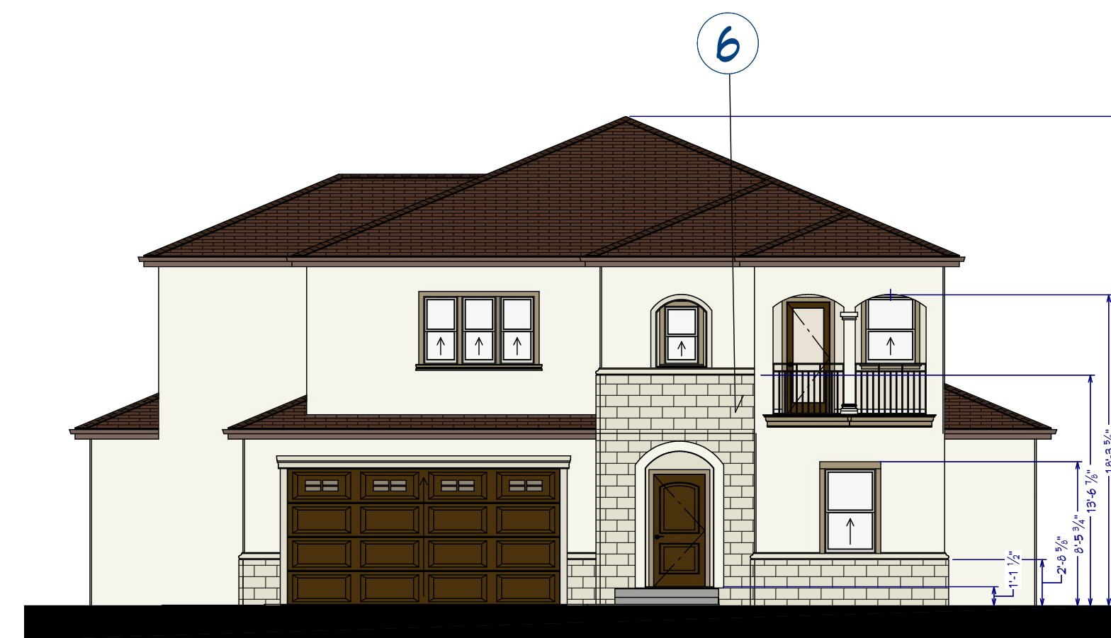
E1 EXTERIOR ELEVATION FRONT 1/8 IN = 1 FT
