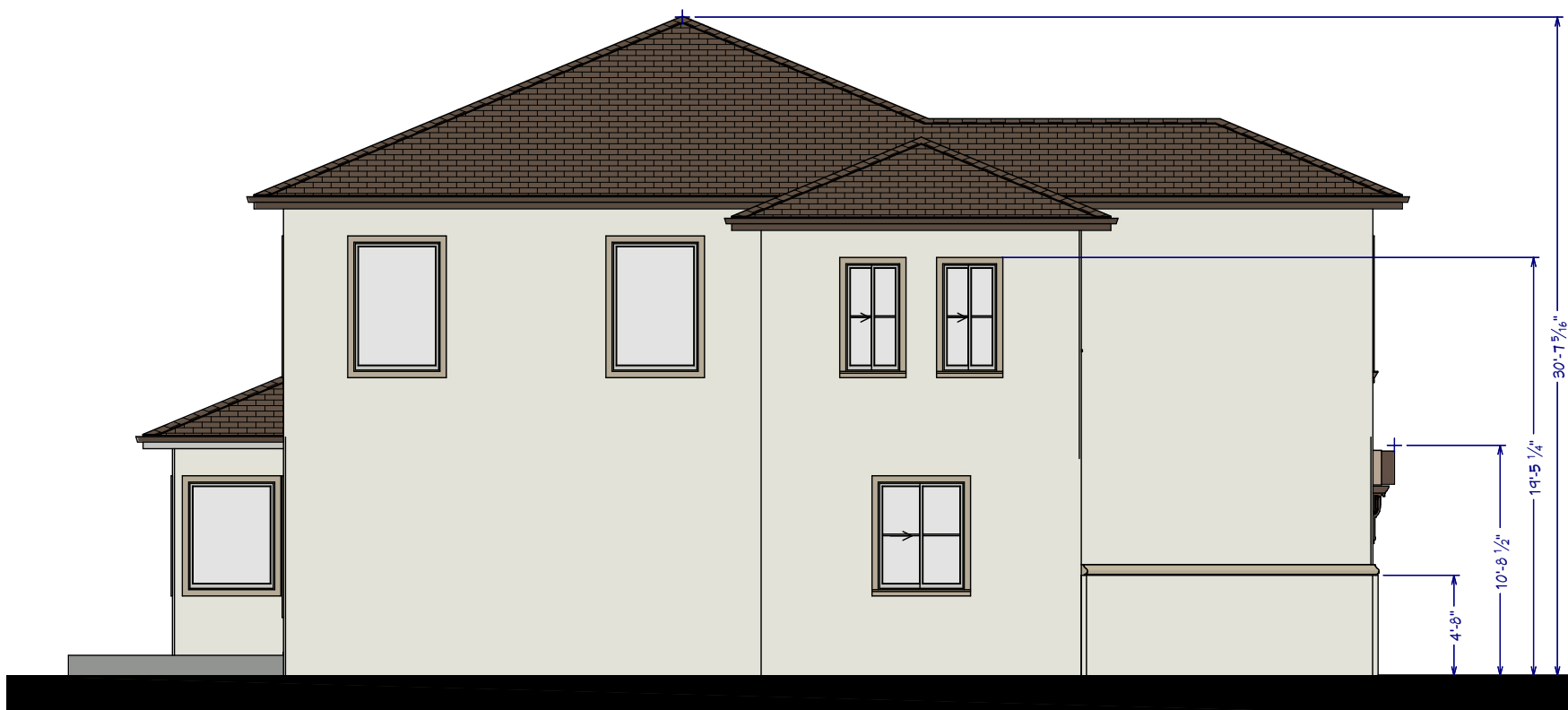
E2 EXTERIOR ELEVATION LEFT 1/8 IN = 1 FT
