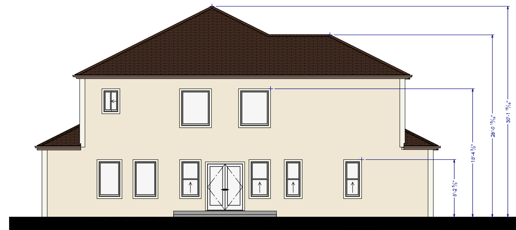
E3 EXTERIOR ELEVATION BACK 1/8 IN = 1 FT
