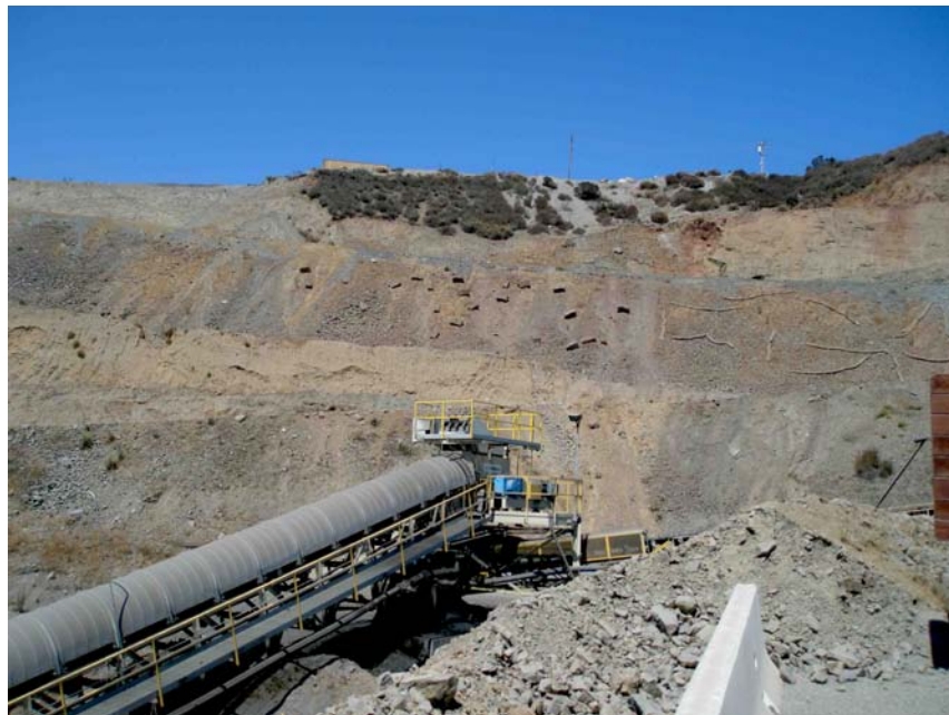
Photo 20: New secondary crusher conveyor dumps to tunnel conveyor, looking north. Note straw bails and waddles on slope. Slope was hydroseeded last winter. Dated September 4, 2014.
