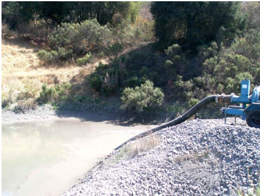
Photo 26: Pond 17 with pump to recycle water back to rock plant. Dated September 4, 2014.
