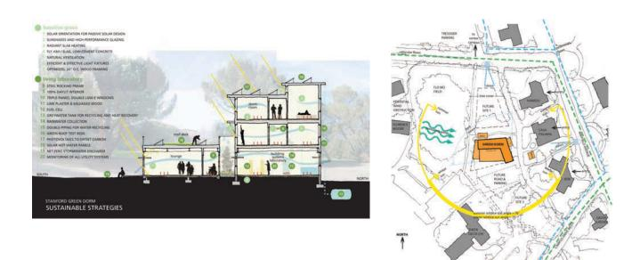
Figure 3.14 Building orientation and site planning to optimize environmental performance
